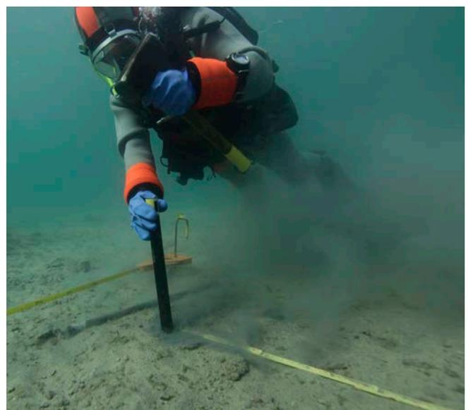
*Fig. 3 Diver placing an erosion marker at Thun, Schadau, Lake Thun. It is a cost-effective and efficient method to measure the erosion rate of the lake bed over the long term © Archaeological Service of the Canton of Bern, Carlos Pinto, 2016.*
